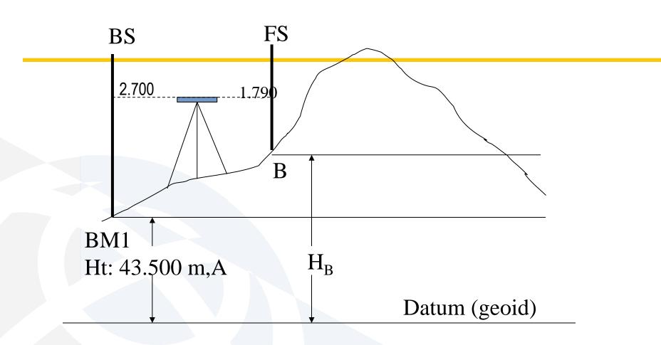
Height of Collimation, HC =  $H_{BM1}$  + BS = 43.500+2.700= 46.200  $H_{B}$  = HC – FS = 46.200 – 1.790 = 44.410
