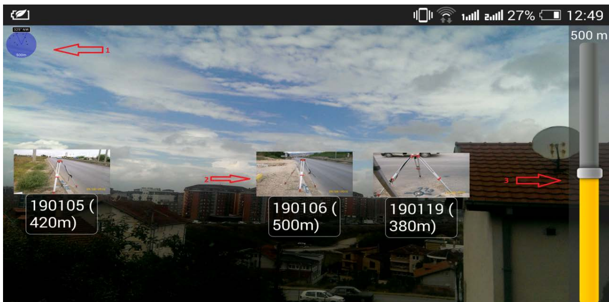
Figure 6. View of third order reference point by device camera (Augmented Reality technology) and other application elements.
