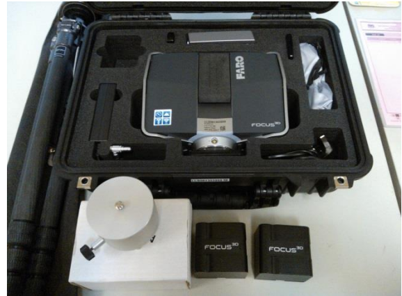
RAJAH 2: Set lengkap peralatan pengimbas laser Faro 3D S
