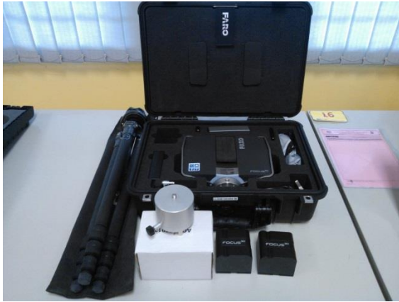
RAJAH 2: Set lengkap peralatan pengimbas laser Faro 3D S
