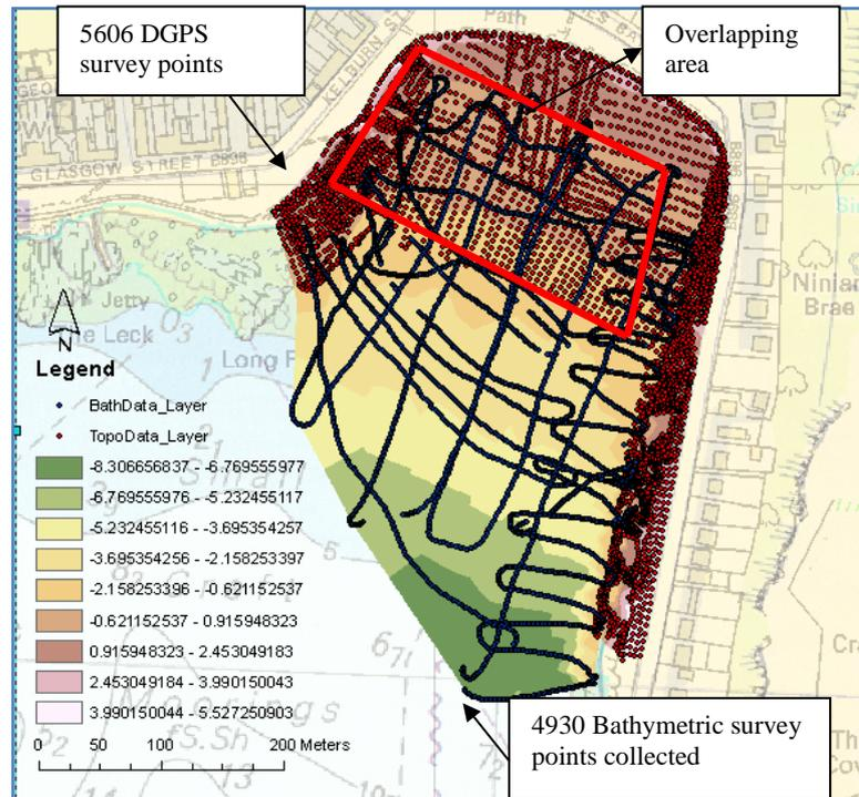
Fig. 2 DGPS and bathymetric surveys carried out at Kames Bay
