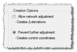
This will cause each point to be created with a Control quality elevation. Only the Control quality elevation will be imported; the observation will not. For the network adjustment, these points will be in the **Fixed Coordinates** list, eligible to be used as fixed points.
