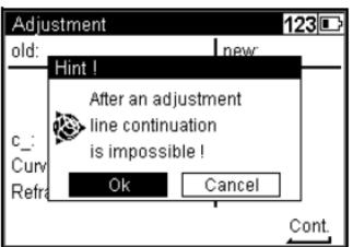
**Note** – After an adjustment is made line continuation is impossible.
