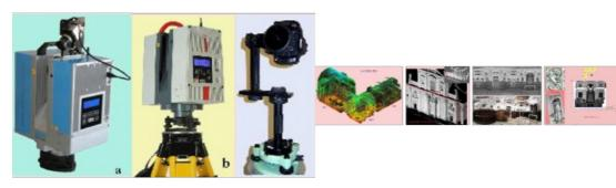
Terrestrial laser scanners are contact-free measuring devices which can collect dense <u>point-clouds</u> of objects. After processing each point is assigned with X, Y, Z coordinates; colour and reflectance value. The relative precision, that is the ratio between absolute precision and measurement range, is better than 10-4.
