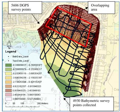
Fig. 2 DGPS and bathymetric surveys carried out at Kames Bay
