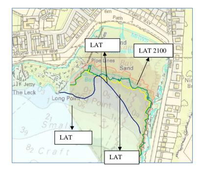
Fig. 5 The shift of LAT position from 1940 to 2100 based on historical data, current survey data and 95% estimates in the high emissions scenario projected by UKCP09
