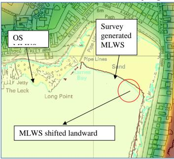
Fig. 3: Comparison of the generated MLWS with the current MLWS shown on OS map.
