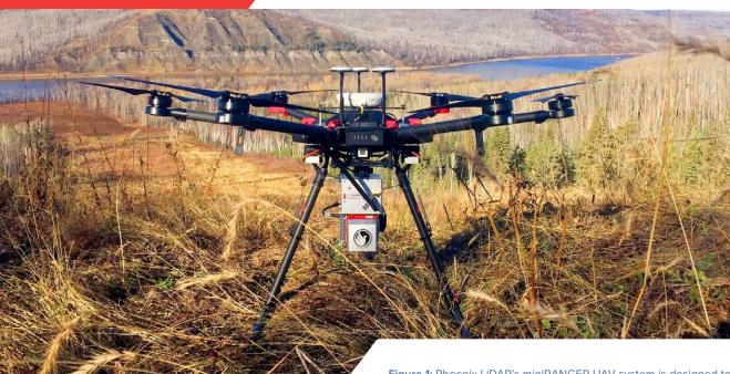
Figure 1: Phoenix LiDAR's miniRANGER UAV system is designed to acquire survey-grade LiDAR data and high-resolution 42 MP RTK photogrammetry at up to 100 meters AGL. This modular system can also be mounted on vehicles and backpacks for more flexibility.
