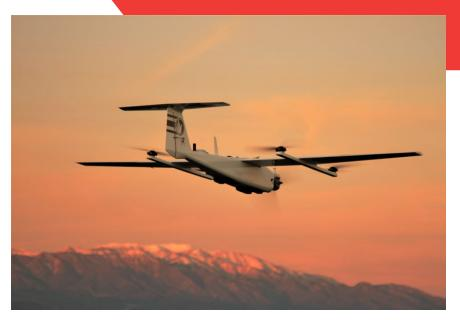
**Figure 7:** The Phoenix TerraHawk CW-20 is a powerful fixed-wing UAV-lidar platform, enabling operators to combine the altitude, stability, and speed of a fixed-wing aircraft with the safety and convenience of a vertical take-off and landing (VTOL) system.
