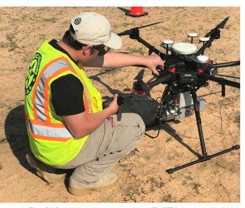
**Figure 6:** A Precision team member prepares their miniRANGER for the mission. Most lidar systems by Phoenix are modular and can be unclipped from their UAVs and mounted onto vehicles, backpacks, and more.
