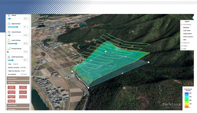
Figure 2: Phoenix Flight Planner enables clients to build flight plans that optimize data collection based on factors such as laser strength, vegetation, terrain, and more. The resulting KMZ can be uploaded for autonomous UAV flight, further simplifying the lidar workflow.
