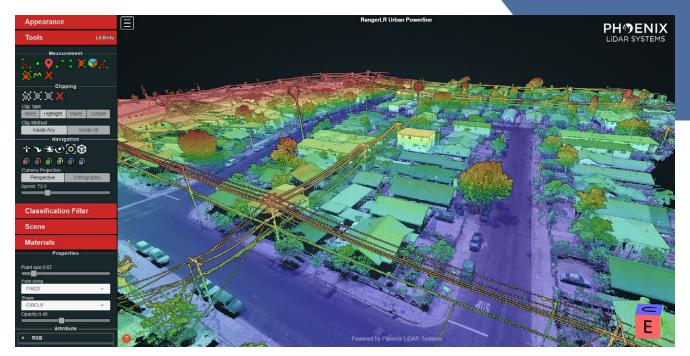
Figure 3: Phoenix LiDARMill produces a smoothed trajectory, automatic flight-line detection, minimization of offsets from overlapping flight lines, and classification of ground/non-ground surfaces. Phoenix believes that it can drive down UAV-lidar costs through LiDARMill's automation and subscription-based cloud service.
